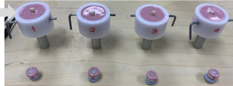
The sectioned tooth was fixed into a composite material in a jig to oppose each different brand of zirconia for comparative wear test.
