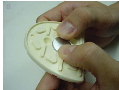
(Insert the metal piece) Push the metal piece into the metal housing plate from the bottom of the plate.
