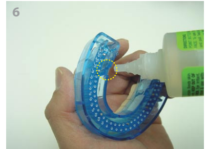
(Glue for the magnet housing) Place a drop of glue in each of the 3 slots located on the bottom of the working tray.
