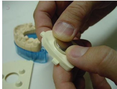
(Insert the magnet) Push the magnet all the way down into the hole on the magnet housing plate .
